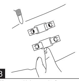
When assembly is secured to frame, proceed to tighening 3 M8 bolts shown below.
