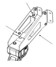
Attach support bracket to through hole with supplied M8 bolt and nut. Tighten to 33ftlbs. Orientation is shown below for driver side, mirror for passenger side. Use the two supplied plastic washers to isolate the bracket and sheet metal to avoid possible corrosion.
