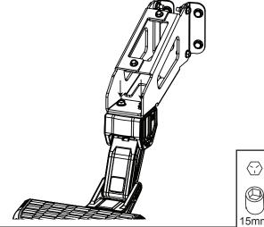
Set assembly in place and tighten 4 M10 bolts (10) to the frame using a 15mm socket. Torque bolts to 33 ft-lbs.
