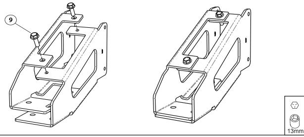
**For 5.5ft Beds, L Bracket Assembly for 5.5ft bed**... On Driver Side, bolt Left Main Bracket (3) to L Bracket (6) and bolt Right Main Bracket (4) to L Bracket (5) using 4 M8 bollts (8). Tighten to 20 ft lbs. For Passenger Side, The L -Bracket will swap postions and orientation.
