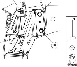
Locate holes on inner fender well and bracket and install support bracket on the inside of front of fender as shown below.
