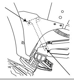
Insert four U clips into cutouts in frame. Be careful not to drop U clips in frame.
