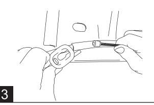
Attach brake cable guide to supplied Brake Cable Bracket (27) and mount bracket with supplied hardware. Reattach brake cable and readjust brake cable adjustment nut to original position.
