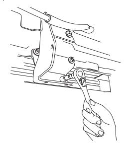
Thread supplied bolts 2x (8) into Front Drive Linkage. Repeat step for Rear Idler Linkage. Do not tighten.
