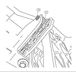
Slide mounting T-nut into position, Center board in rail pocket. Tighten fasteners to 10 ft-lbs.
