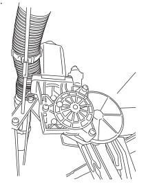
Torque bolts on mounting brackets to 16ft-lbs.
