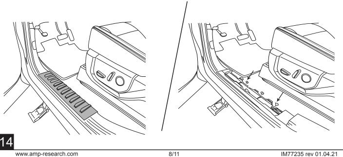
Remove grommet in floor panel above front linkage on driver side. Poke small hole into grommet and thread the two trigger wires through and up into the cabin of vehicle. Seal grommet with silicone sealer.
