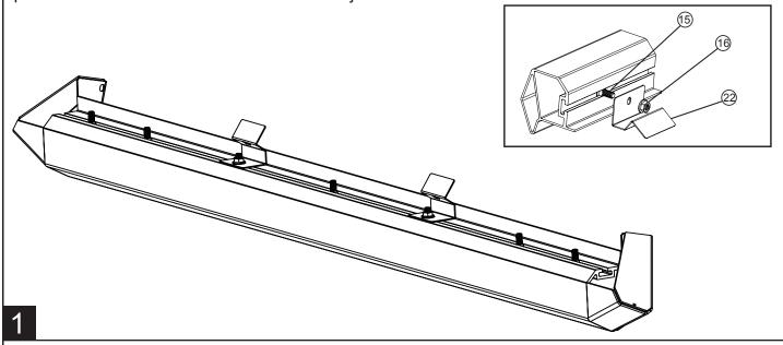
Using Flange Nuts (16), assemble Brackets 2x (24) & 1x (25) onto the Rail (4), using the Carriage Bolts (15) left from previous step. Next, install Flange Bolt (13) and Flange Nut (16) onto bracket tab. Driver side shown. Dimensions shown are for reference.
