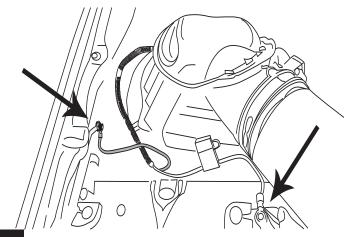
Route factory harness underneath vehicle and plug in motors (both sides). Route remaining LED light wires back towards rear of vehicle.
