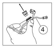
Attach wire harness to controller (make sure connector locking tabs fully engage). Mount controller with the two 11" tie wraps to factory conduit, just forward of battery.
