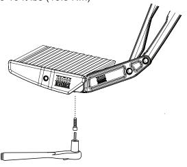
On each side of the vehicle measure from the rear linkage to end of the board. Measurement should be approximately 11" as shown below.
