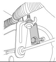
Locate mounting points; first and last set of studs on the inner sill.
