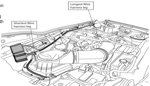
Attach harness ground to body ground located on inner fender. Connect red leads to positive terminal on battery.
