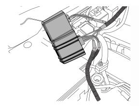
Route shorter leg of harness down passenger-side wheel well and longer leg of harness down along driver side wheel well. Secure with tie wraps.
