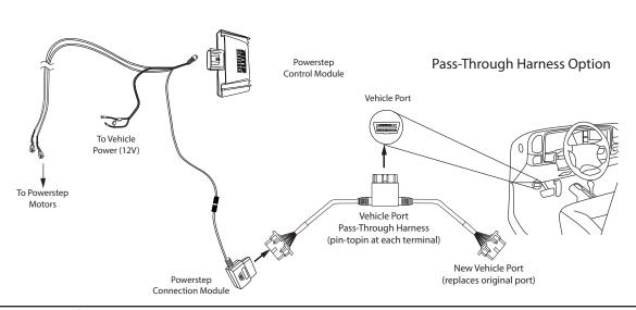
Route the two Wire Harness legs down over the wheel wells toward Motor Linkages, long leg across to the passenger side.
