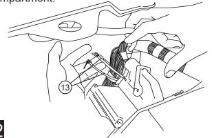
Insert controller into tie-wrap loops and cinch down securely. The tie-wraps should cinch down into channels on controller surface.
