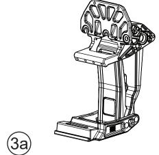
Idler Linkage Assembly - Driver Side
