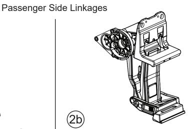
Motor Linkage Assembly - Passenger Side
