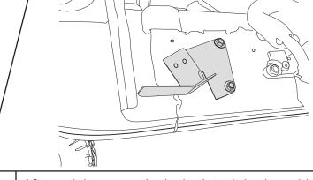
While holding brake cable adjustment nut with wrench (located on driverside along frame, towards the rear), loosen brake cable to allow
