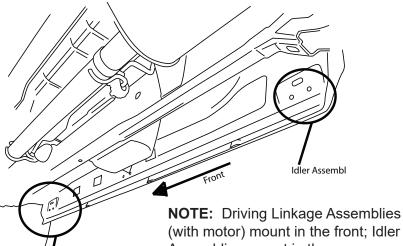
(with motor) mount in the front; Idler Assemblies mount in the rear.
