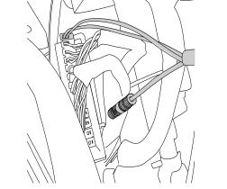
Secure harness with supplied tie wraps. Make sure wires are away from E-brake mechanism and brake pedal assembly.
