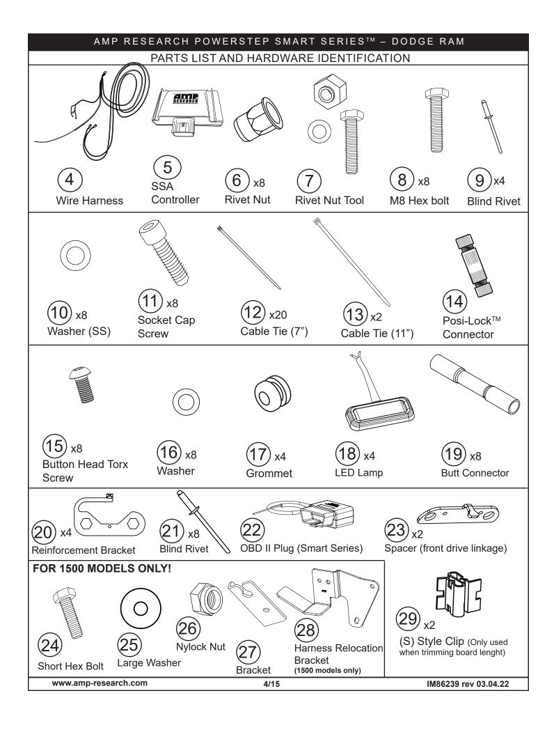
NOTE: 1500 RAM Only! Powerstep installations require additional steps and come with the required additional hardware. Please read and carefully follow the **instructions on page 1.** Follow Steps 1-5 to relocate brake cable and wire harness plug and then proceed with the Power Step installation. For Ram 2500/3500 Skip to step 6.
