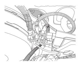
Tape leading end of wires together and push through rubber boot to cabin side of the firewall. Silicon lubricant may be used for ease of passage. The trigger wires will come out just above and to the left of the brake pedal.
