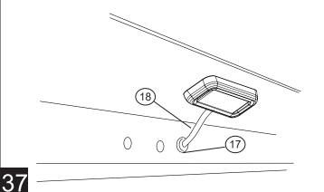
Close and wrap with conduit and electrical tape. Secure all loose wires with cable ties, with lamp wires pulled upward to avoid any wire snagging.
