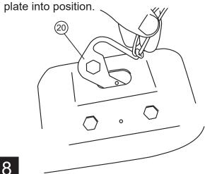
Set rivet nuts into place for alignment. Insert pop rivet through hole in plate and secure in place. Once pop rivet is installed remove string or wire from Reinforcement Plate. NOTE: Verify plate is pulled flush to the body before securing pop
