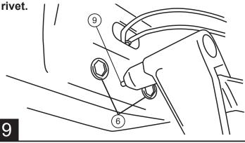
Assemble Rivet Nut Tool (Hex Bolt (lubricated with soapy water), Washer, Rivet Tool) (7), and Rivet Nut (6) together as shown and place into hex cutouts in sill. An extra Hex Bolt and M8 Washer is supplied to install rivet nuts.
