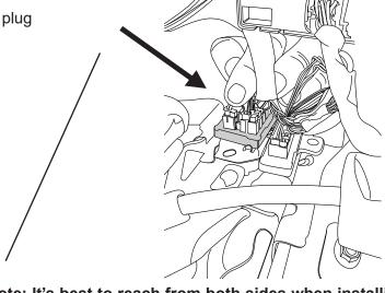
Note: It's best to reach from both sides when installing 2 pin plug. Any open port on green plug can be used.
