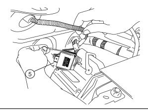
Remove fuses from Power Step Wire Harness.
