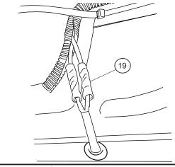
Drill a 9/32" hole through the pinch weld at marked locations. Debur all holes. After drilling apply paint to holes to prevent rusting.
