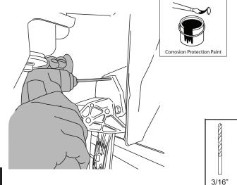
Using a Rivet Gun install rivets (21).
