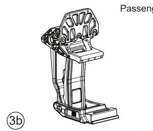
Idler Linkage Assembly - Passenger Side
