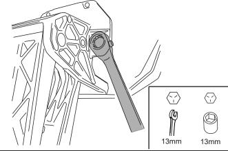
If crash bracket is not present use supplied spacer in place of bracket. Spacer can be inserted after linkage is up into position. Spacer will be held in place by drilling and pop riveting into place. Rivets will be installed in step 41 & 42.
