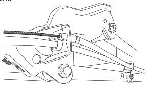
Attach brake cable guide to supplied Brake Cable Bracket (27) and mount bracket with supplied hardware (24,25,26). Reattach brake cable and readjust brake cable adjustment nut
