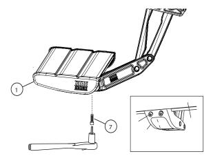
On each side of the vehicle measure from the rear linkage to end of the board. Measurement should be approximately 11" as shown below.
