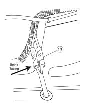
Close and wrap with conduit and electrical tape. Secure all loose wires with cable ties with lamp wires pulled upward to avoid any wire snagging.
