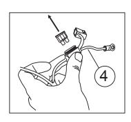
Attach wire harness to controller (make sure connector locking tabs fully engage). Mount controller with the two 11" tie wraps (15) to factory conduit, just forward of battery.
