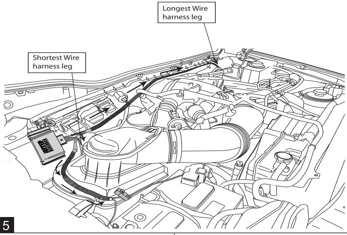
Attach harness ground to body ground located on inner fender. Connect red leads to positive terminal on battery.
