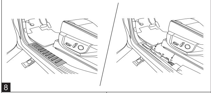
On Crew Cab models, remove grommet in floor panel above front linkage on driver side. Poke small hole into grommet and thread the trigger wire through and up into the cabin of vehicle. Seal grommet with silicone sealer.
