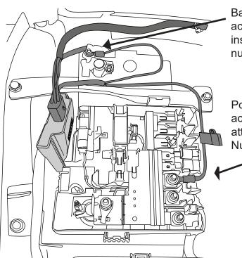
Battery terminal accessory stud, install under factory nut.
