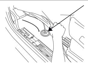
On the Driver side, Do Not zip tie the Wire Harness to the Brake Lines.
