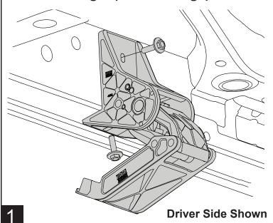
Install the Idler linkage in the **First mount position at the front of the truck**, for Passenger and Driver sides, using the conical washer bolts (13). All plastic or rubber hole plugs need to be removed that are next to the linkage mounts. Also, an extra vertical seam-sealer bead may need to be removed from the front linkage mounting surface.
