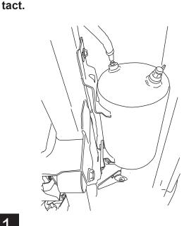
Mount Front and Rear Bracket. Rear bracket will Re-Use hardware removed in step 1. Front bracket will use provided flat head screw(6).
