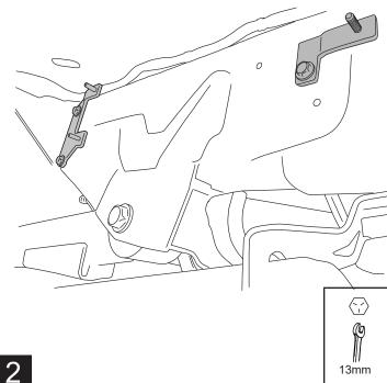
Set tank into position and tighten 3 nuts holding tank to relocation brackets.
