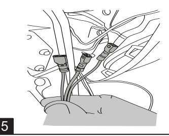
Mount controller with the two tie wraps provided. . Route override switch harness across firewall and into the cab of vehilce.
