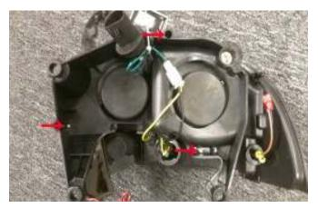
On the back side of the light there are 3 adjustment screws. You can turn these screws to move the bracket closer to the housing. by doing this you will be able to adjust the gap between the fenders and the light. You may have to take the light out a couple times and adjust the screws to get the desired gap.
