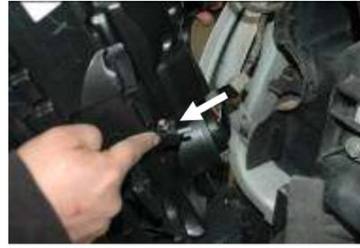
You can adjust the level of the light by adjusting the screw located directly above the Anzo headlight housing.
