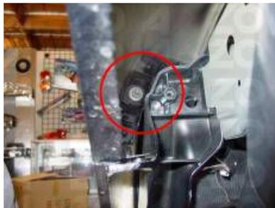
Step 6: Remove the 10mm bolt located inside the fender behind the headlight housing.
