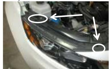
Remove (2) 10mm bolts located on top of the headlight
