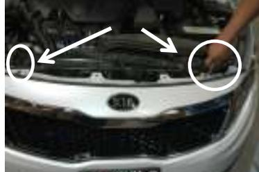
Remove (2) 10mm bolts located on each side of the bumper
