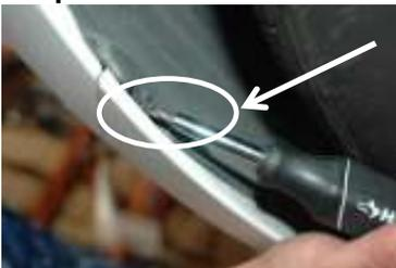
Remove (1) screw located on each side of the fender wall
