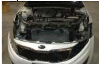
Before removing the bumper remove (1) 10mm bolt followed by push pins located underneath the bumper
