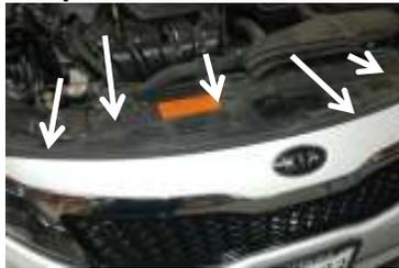
Remove push pins located on top of the plastic cover
