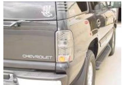
Step 8: Put the tail light in and screw in the two screws to hold the tail light in place.
