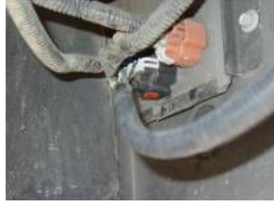
Step 1: Locate the main circuit board for the tail light underneath the vehicle located in the passenger rear.
