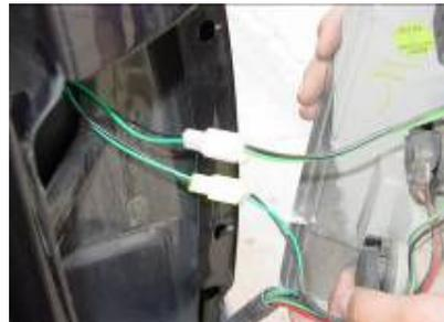
Step 7: plug the two resistors into the tail light.
