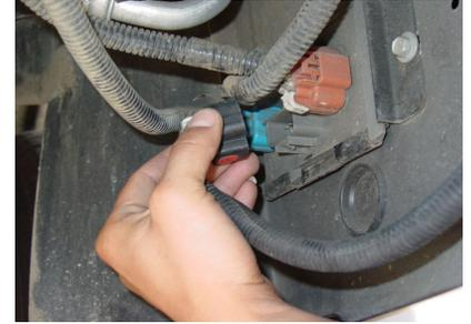
Step 2: Unplug the middle wire harness from the circuit board.
