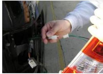
Step 8: Plug the resistor to the taillight.
