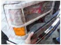
Step 2: Remove the parking lights from the vehicle.
