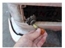
Step 4: Twist off the bulb from the socket.
