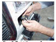
Step 5: Twist the new Anzo parking light bulb connector to the socket.
