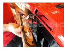
Step7: Twist the two cargo blubs into the new Anzo light.
