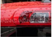
Step 1: Locate the two phillips screw on both ends of the third brake light and remove
