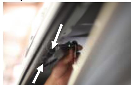
Remove the two 10mm bolt located
