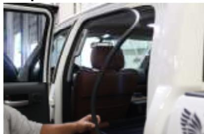
Remove the rubber molding
