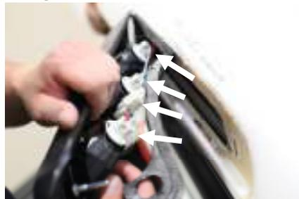
Remove the third brake light by disconnecting the power source and the three light bulb harnesses
