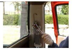
Use the 14mm socket to remove the bolt holding in the seat belt.
