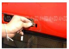
Put in the supplied screw holder on to the original hole for the bolts.
