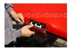
Pull out the 3rd brake light from the vehicle.
