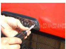
Use the supplied screws to install the new led 3rd brake light.
