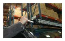
Once you have the bar installed go through and tighten all the bolts down.
