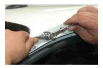
Place your 1/2 wrench on the nuts and your 7/16 wrench on the hex bolt. You will want to keep the nuts from spinning as you tighten the hex bolt which will crush the grip sert against the body.
