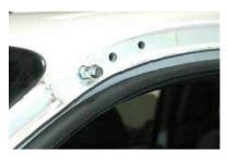
Once your holes are drilled insert the grip sert into the hole you will need to tap it in as it is a snug fit. Next install the 1/4 - 20 hex bolt washer and 2 nuts in the grip sert.
