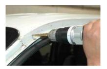
Make sure when drilling your holes you keep your drill straight starting with a smaller bit or a universal bit start drilling. The final size of the hole will be 3/8 inch.
