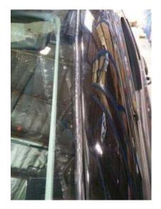
We have found that running the wires down the channel in-between the glass and the pillar is the best place. You can push the harness down with minimal pressure and the harness will stay in place.
