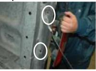
Remove the passenger side tail light by removing the two 8mm
