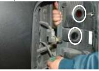
Remove the reverse and the brake light bulbs from its sockets.
