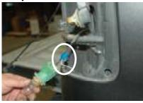
Splice the white Anzo Spoiler power source wire to the red reverse light power source wire.
