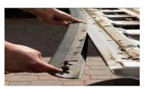
Remove your stock cap by pulling up from one corner. The cap is held in with clips so you may need to use some force to get it started.
