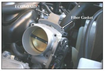
4. Install the ECONOAID Throttlebody Booster against the intake manifold with the logo facing the throttlebody. Next install the supplied gasket between the ECONOAID and the throttlebody.
