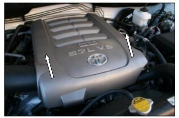
1. <u>Disconnect the negative battery cable!</u> Lift up on the front of the engine beauty cover, and then remove it from the vehicle.
