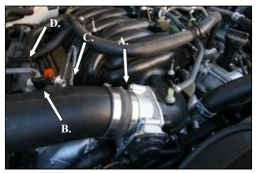
**2. A.**) Loosen two hose clamps, one at the air box, and one at the throttlebody. **B.**) Squeeze the tab on the electrical connector and disconnect it from the Mass Air Sensor. **C.**) Disconnect the 1/8" vacuum line from the air intake tube. **D.**) Disconnect the crankcase breather hose from the intake tube. Remove the air intake tube from the vehicle.
