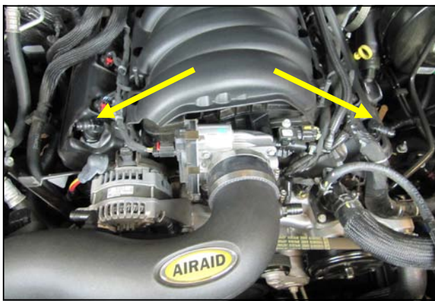
10. Install the supplied Quick Connect Fittings on to the valve cover breather fittings.
