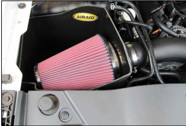
13. Install the Airaid Premium filter onto the Filter Adapter , and tighten the hose clamp.
