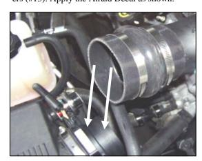
**10.** Install the urethane hump hose (#6) onto the Airaid Intake Tube (#5) and the MAF sensor with two #60 hose clamps (#15). Install the tube assembly onto the engine. (Hint: slide the hump hose all the way onto the end of the tube.)
