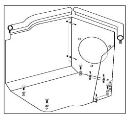
**6.** Assemble the Airaid Cool Air Dam panels (#2, #3) using five 6-32x 5/16" screws (#9), #6 flat washers (#10), and 6-32 keps nuts (#11).
