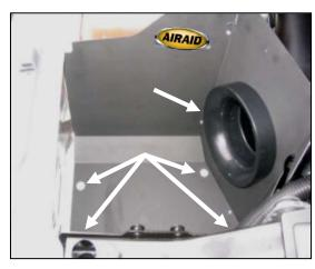
7. Install the air filter adapter (#4) using three <sup>1</sup>/<sub>4</sub>-20x 1/2" button head bolts (#12), and 1/4" flat washers (#13). Position the Airaid Cool Air Dam in place of the factory airbox & secure it with four M6-1x25 hex bolts (#14) and 1/4" flat washers (#13). Apply the Airaid Decal as shown.
