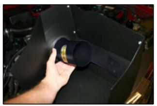
**4.** Insert the Airaid intake tube (#5) thru the hole in the **MAF** panel and then rotate it clockwise so that the holes in the bracket on the tube line up with the two holes in the bottom panel. Apply the Airaid Decal onto the Intake Tube as shown.
