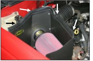
8. Install the Airaid Premium Filter (#1) onto the Airaid intake tube as shown, and then tighten the hose clamp. Next, install the weather strip on top of the CAD, starting at the right fender working your way towards the front of the vehicle.
