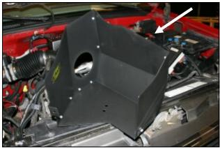
**2.** Assemble the three Cold Air Dam (CAD) panels (#s 2, 3, &4) as shown using nine 6-32 screws (#10), nine #6 washers (#9), and nine nuts (#11). Apply the Airaid Foil Decal onto the Panel as shown.
