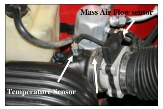
1. **Disconnect the negative battery cable. VERY CAREFULLY!** Remove the air intake temperature sensor first, and then the grommet from the air intake tube and set them aside. *There is no need to disconnect the wiring harness on the temp sensor.*Loosen the hose clamp that secures the air intake tube to the **Mass Air Flow (MAF)** sensor.
