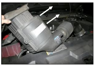
**2.** Rock the air filter housing back and forth while lifting up, and remove the factory intake assembly from the vehicle. There are only grommets holding it in place.
