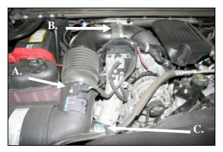
1. Disconnect the negative battery cables. A.) Using a #20 Torx bit remove the two screws and the Mass Air Flow sensor from the factory intake tube.
