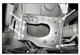
3. Using a 10mm socket, remove 4 bolts, and remove the factory air filter mounting plate.
