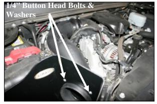
6. Slide the Airaid Intake Tube (#2) into the CAB first, and then into the hump hose. If needed, the factory turbo intake tube can be adjusted for proper alignment. Next install four 1/4" button head bolts (#6), and four flat washers (#7) thru the CAB to secure the Airaid Intake Tube. Now tighten the three bolts at the bottom of the CAB and the two hose clamps on the hump hose.
