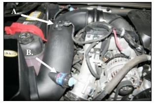
7. A.) Reinstall the Mass Air Flow sensor into the Airaid Intake Tube using two 8-32x 3/8" button head screws (#8). <u>Do Not Use The Factory Screws!</u> It may be necessary to reroute the MAF sensor wiring
