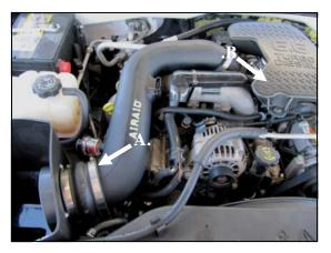
14. A.) Install the hump hose end of the Airaid intake tube assembly onto the filter adapter first. **B.**) Slip the coupler end of the tube over the factory turbocharger inlet. Adjust for fit, and tighten the hose clamps
