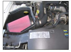
**15.** Install the Airaid Premium Filter (#1) onto the filter adapter, and tighten the hose clamp. Install the weather strip (#7) onto the Airaid Cold Air Box. Reconnect the M.A.F. sensor . Apply the Airaid Decal inside of the Airbox as shown.
