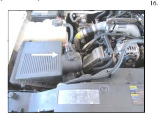
2. Disconnect the Mass Air Flow (M.A.F.) sensor and remove the factory airbox. Rock the factory air box back and forth and remove it from it's mounting. It is held in place with grommets.
