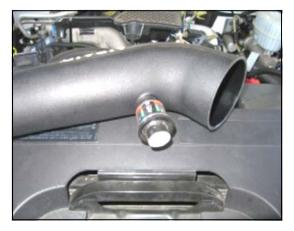
9. Transfer the factory rubber grommet and air filter minder from the airbox top into the Airaid intake tube As shown.
