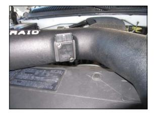
8. Transfer the M.A.F. Sensor from the factory airbox into the Airaid intake tube (#2). Use the two 8-32 button head screws (#10). to secure the meter. Do Not Use Factory Screws.
