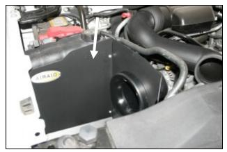
7. Install the assembled **CAD** into the vehicle where the mounting plate was removed in step #4. Secure the CAD to the vehicle using four 6mm bolts (#12) and four flat washers (#11). Do not over tighten the bolts.
