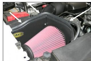
**9.** Install the Airaid Premium Filter (#1) onto the filter adapter and tighten the hose clamp. Next install the weather strip (#5) onto the top of the **CAD** as shown. Start at the right fender and work your way around towards the radiator.
