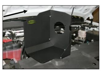
**5.** Assemble the two Cold Air Dam (CAD) panels (#2 & #3) using five 6-32 Phillips screws (#6) five flat washers (#7), and five keps nuts (#8) as shown. Make sure that panel #2 is located inside of panel #3. Apply the Airaid Foil Decal onto the Panel as shown.
