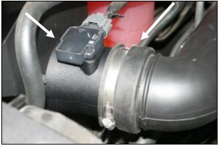
**8.** Reinstall the **MAF** sensor onto the filter adapter using two 8-32 x 5/8" button head screws (#9).
