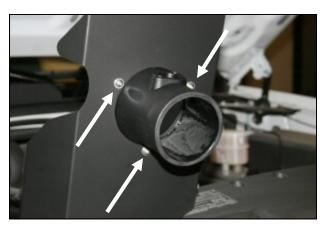
**6.** Install the filter adapter into panel #3 as shown, using three  $1/4-20 \times 1/2$ " button head bolts (#10), and three flat washers (#11).
