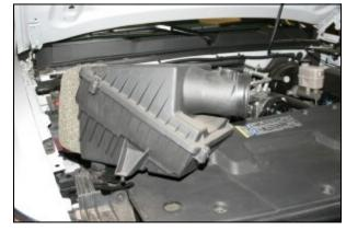
**3.** Rock the factory airbox back and forth while lifting up on it, and remove it from the vehicle. It is only held in place by grommets.
