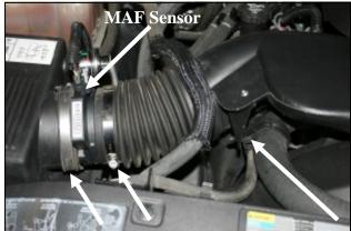
Loosen two hose clamps. One on each side of the Mass Air Flow (MAF) sensor.
