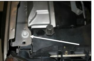
**7.** Remove the factory bolt that secures the right front fender to the radiator support. It will be reused in step #8.
