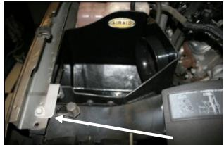
**8.** Install the **CAB** assembly into the vehicle where the factory airbox used to be using three 6mm hex bolts (#12) and three flat washers (#11) thru the bottom. Now reinstall the factory fender bolt thru the bracket and into the fender. Adjust the assembly for fit and tighten all bolts and nuts at this time. Apply the Airaid decal inside the Airbox as shown.
