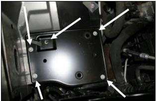
**5.** Using a 10mm socket, remove the bolts that secure the factory air filter housing platform and remove it from the vehicle.
