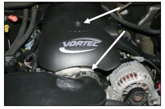
1. **Disconnect the negative battery cable.**Loosen the bolt that secures the beauty cover to the engine and remove it and the cover from the vehicle.
