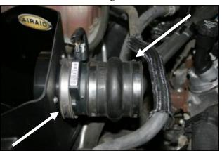
**9.** Reinstall the **MAF** sensor and coupler onto the filter adapter and tighten the clamp.
