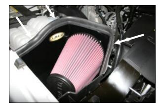
**8.** The Airaid Premium filter (#1) is a very tight fit in the **CAB**. For ease of installation, hold the filter in your right hand, and guide the bottom of the filter past the flange of the tube with your left hand inside of the **CAB**. It will fit! Tighten the hose clamp. Next install the weather strip (#5) on top of the **CAB**, starting at the fender and working your way towards the radiator.
