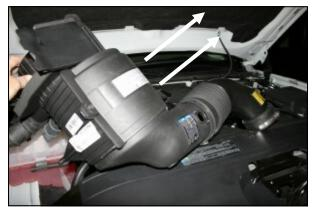
**2.** Rock the air filter housing back and forth while lifting up, and remove the factory intake assembly from the vehicle. There are only grommets holding it in place.
