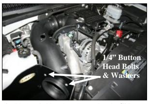
**6.** Slide the Airaid Intake Tube (#2) into the **CAB** first, and then into the hump hose. *If needed, the factory turbo intake tube can be adjusted for proper alignment.* Next install four 1/4" button head bolts (#6), and four flat washers (#7) thru the **CAB** to secure the Airaid Intake Tube. Now tighten the three bolts at the bottom of the **CAB** and the two hose clamps on the hump hose.
