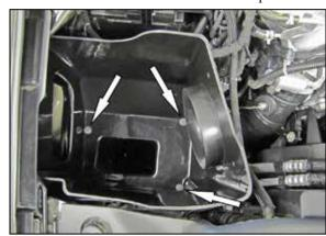
6. Install the AIRAID® Cold Air Box into the vehicle and secure to the air filter mounting plate location and secure with three of the factory bolts from step #4.
