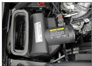
3. Release the red locking tab and then disconnect the mass air sensor electrical connection. Unhook the coolant bypass hose from the air box. Lift the factory air filter housing up to dislodge it from the mounting grommets and then remove the housing from the vehicle.
