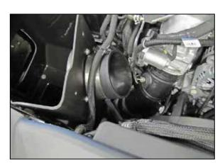
7. Install the elbow coupler hose clamps onto the filter adapter as shown but do not tighten at this time.
