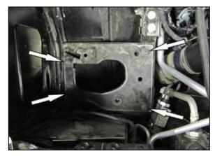
4. Remove the four bolts that secure the air filter mounting flange to the inner fender and then remove the mounting flange from the vehicle.
