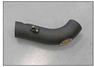
9. Install the mass air sensor into the AIRAID® intake tube and secure with the provided hardware. Install the AIRAID® decal to the tube.
