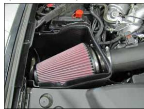
13. Install the weather strip onto the edge of the Cold Air Box so the contour rolls away from the air filter. NOTE: Some trimming of the weather strip will be necessary. Install with lip rolling away from the filter.
