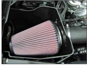
12. Using care so as not to damage the air filter, Install the AIRAID® air filter into the air box and onto the filter adapter, then secure with the provided hardware.
