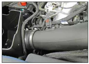
11. Reconnect the mass air sensor electrical connection, clip the coolant bypass hose to the AIRAID® Cold Air Box using the factory retaining clip.
