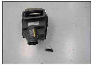
8. Remove the mass air sensor from the factory air filter housing as shown.
