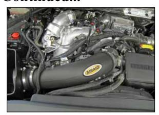
10. Install the AIRAID® intake tube into the elbow coupler and then into the factory plenum, adjust the elbow coupler and intake tube for best fit and then secure with the provided hose clamps.
