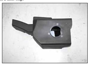
5. Install the provided air filter adapter into the AIRAID® Cold Air Box and secure with the hardware provided.
