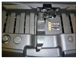
29. Reinstall the hood release arm to the hood latch and secure with the factory bolts.
