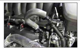
3. Depress the locking tabs and then disconnect the crank case vent line from the intake plenum and valve cover vent port.
