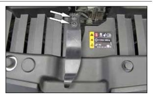
5. Remove the two bolts that secure the hood release arm to the hood latch and then remove the release arm.
