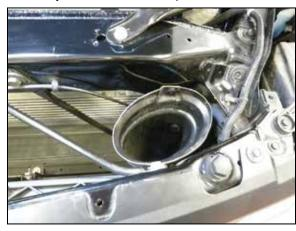
14. Push the factory fresh air intake duct into the AIRAID® air filter housing and then reinstall the plastic clip to secure it into position.
