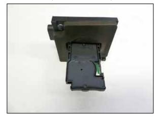
18. Install the provided gasket onto the provided mass air sensor adapter. Remove the mass air sensor from the factory air filter housing and then install it into the adapter and secure with the provide hardware.
