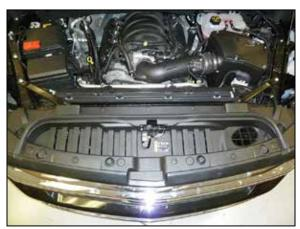
28. Reinstall the upper radiator valence and secure with the factory retaining clips.
