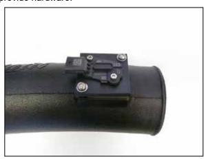
19. Install the mass air sensor assembly into the AIRAID® intake tube in the direction shown and secure with the provided hardware.
