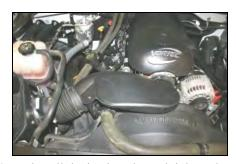
**10.** Re-install the intake tube and tighten the hose clamps. Re-install the plastic holder from step #1.
