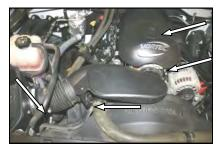
1. <u>Disconnect the negative battery cable!</u> Loosen one bolt and remove the beauty cover. Pry the tube from the clamp on the radiator hose. Loosen the hose clamps on each end of the intake tube and remove the tube.
