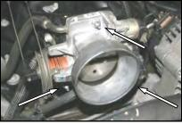
**2.** Using a 10mm socket, remove the three nuts that hold the throttle body to the intake manifold.
