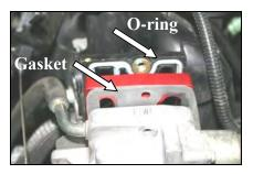
6. Place one fiber gasket (#4) between the Airaid spacer (#1) and the throttle body. Make sure the flat face of the Airaid spacer is against the throttle body with the bore extending into the intake manifold. Use caution to retain the factory o-ring gasket on the intake manifold.
