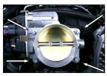
**3.** With a 10mm socket remove the two nuts, and the two bolts that hold the throttle body to the intake manifold. Without disconnecting the wiring harness, set the throttle body aside.
