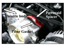
5. Install 2 of the supplied bolts (#2) and washers (#3) thru the two holes in the top of the throttle body, thru the supplied fiber gasket (#4), thru the Airaid Spacer, and into the two brass inserts in the intake manifold. Run the bolts in a few threads with your fingers. Use caution not to cross-thread the bolts. Next install the 2 remaining bolts (#2) and washers (#3) in the two bottom holes of the throttle body, and tighten in a cross pattern to the vehicle manufacture's specifications.
