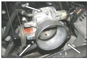
2. Using a 10mm socket, remove three nuts on the throttle body.
