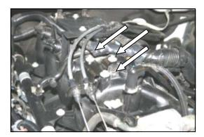
4. Using a 5/16" socket, remove and save the three bolts that hold the throttle cable bracket to the intake manifold.
