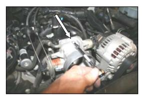
3. Using a 4mm socket, remove the three studs that hold the throttle body to the intake manifold. No need to remove the throttle body, leave it hang where it is.
