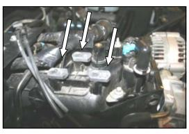
5. Install the three linkage plates (#5) with the three flat head screws (#6) as shown, pointing towards the front of the vehicle.
