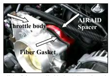
5. Install 2 of the supplied bolts (#2) and washers (#3) thru the two holes in the top of the throttle body, thru the supplied fiber gasket (#4), thru the AIRAID Spacer, and into the two brass inserts in the intake manifold. Run the bolts in a few threads with your fingers. Use caution not to cross-thread the bolts. Next install the 2 remaining bolts (#2) and washers (#3) in the two bottom holes of the throttle body, and tighten in a cross pattern to the vehicle manufacturer's specifications.
