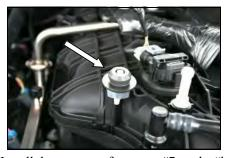
**8.** Install the grommet from step #7 on the "ball stud", with the small diameter facing up as shown.
