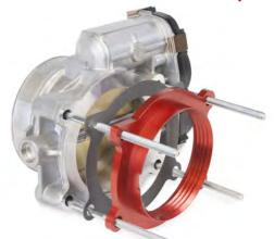
Example of proper spacer installation. Spacer must protrude into intake manifold and away from throttle body.
