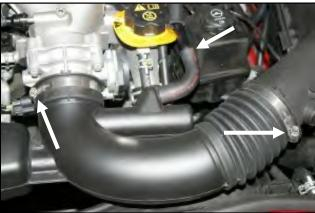
2. Disconnect the breather hose elbow at the hard plastic breather tube. Loosen the two hose clamps that secure the intake tube to the throttle body, and the air cleaner lid. Remove the air intake tube.
