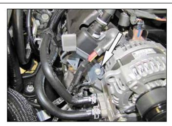
2. On vehicles equipped with a intake plenum support brace secured to the passenger side cylinder head, remove the bolt shown securing the support bracket.
