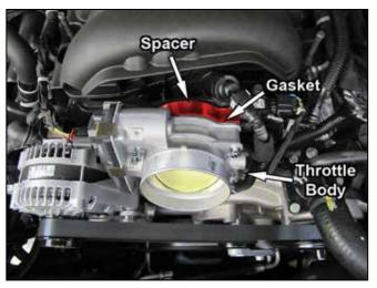
5. Install the provided new bolts through the holes in the throttle body, through the holes in the provided gasket and through the AIRAID spacer. Start the new bolts into the inserts in the intake manifold being careful not to cross thread the bolts. Tighten the bolts in a cross pattern to the factory specifications.
