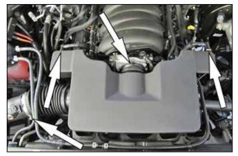
1. **Disconnect the negative battery cable!** Disconnect the crank case vent line quick disconnect fittings from the intake plenum. Loosen the two hose clamps that secure the intake plenum to the throttle body and to the air filter housing, then remove the intake plenum from the vehicle.
