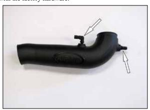
6. Install the provided  $90^{\rm o}$  and straight vent fittings into the AIRAID<sup>®</sup> intake tube as shown.
