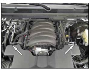
2. Disconnect both crank case quick connect vent lines from the valve covers.
