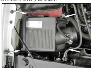
4. Loosen the screws that secure the upper air filter housing and then lift off the housing to remove the factory air filter.
