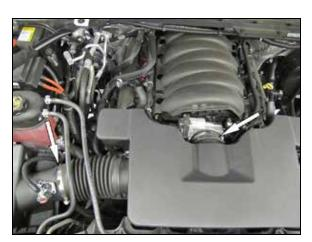
3. Loosen the hose clamps that secure the intake plenum to the throttle body and air filter housing. Then remove the intake plenum from the vehicle.
