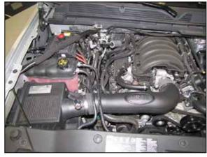
13. Double check your work!Make sure there is no foreign material in the intake path.Make sure all clamps, hoses, bolts, and screws are tight.Double check the hood clearance!Reconnect the negative battery cable!
