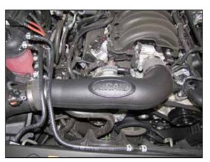
10. Install the AIRAID<sup>®</sup> intake tube into the coupler on the air filter housing and then onto the throttle body, adjust the tube for best fit and then secure with the provided hose clamps.
