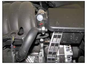
2. Disconnect the crank case vent quick connect fitting from the factory intake plenum.
