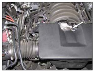
4. Loosen the hose clamps securing the intake plenum to the throttle body and air filter housing then remove the intake plenum from the vehicle. **NOTE: Airaid recommends that customers do not**
