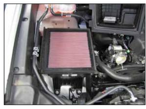
5. Install the AIRAID® air filter and then reinstall the upper housing and secure with the factory screws.
