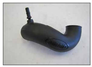
7. Install the provided vent fitting into the AIRAID® intake tube as shown.
