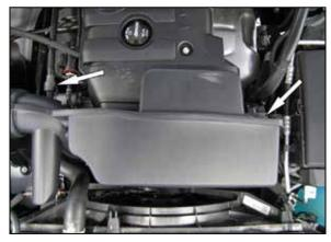
3. Disconnect the crank case vent line from the intake plenum and remove the bolt that secures the plenum to the engine. Remove the intake tube and plenum from the vehicle.
