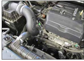
9. Install the intake tube into the coupler at the throttle body, align with the coupler on the air filter housing. Adjust the tube for best fit and secure with the provided hose clamps. Reconnect the crank case vent line.
