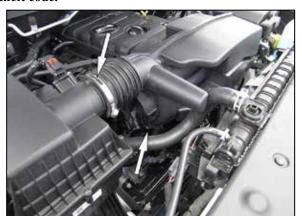
2. Loosen the hose clamps that secures the intake tube to the air filter housing and to the throttle body.
