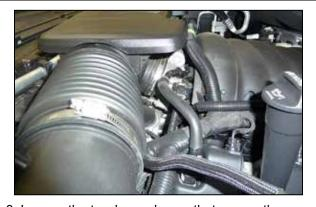
3. Loosen the two hose clamps that secure the intake plenum to the throttle body and the air filter housing and then remove the intake plenum from the vehicle.
