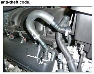
2. Depress the locking tabs and then remove the crank case vent hose assembly.
