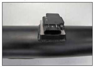
9. Remove the two screws securing the mass air sensor to the air box and then remove the mass air sensor from the air box as shown. Install the mass air sensor into the AIRAID<sup>®</sup> intake tube and secure with the provided hardware.
