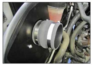
19. Install the provided hump coupler hose onto the filter adapter and secure with the provided hose clamp.
