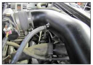
23. Install the provided crankcase vent hose onto the valve cover vent port and then connect the remaining open end to the  $\frac{1}{4}$ " NPT fitting in the AIRAID<sup>®</sup> intake tube.
