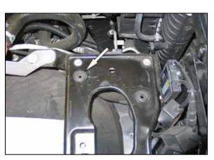
12. Remove the air box mounting grommet shown from the air box mounting plate.
