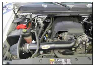
**26.** Double check your work! Make sure there is no foreign material in the intake path. Make sure all clamps, hoses, bolts, and screws are tight. Double check the hood clearance! Reconnect the negative battery cable!
