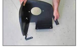
16. Reinstall the heat shield assembly onto the air box mounting plate and secure the two 5/16" bolts provided.
