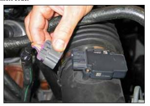
2. Disconnect the mass air electrical connection.
