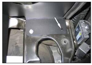
14. Set the heat shield assembly into position with the inserted nut installed into the air box mounting grommet location. Mark the heat shield mounting location to be drilled.
