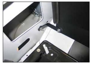
17. Secure the mounting bracket to the inner fender with the hardware provided.
