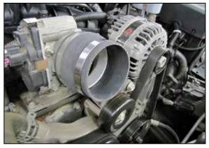
20. Install step coupler hose onto the throttle body and secure with the provided hose clamp.
