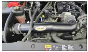
22. Install the AIRAID<sup>®</sup> intake tube into the silicone hose at the filter adapter and then into the silicone hose at the throttle body, then secure with the provided hose clamps.
