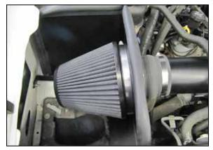
24. Install the AIRAID<sup>®</sup> air filter onto the filter adaptor and secure with the provided hose clamp.
