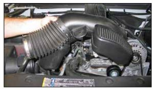
6. Loosen the hose clamp which secures the stock intake tube, then remove the intake tube from the vehicle.
