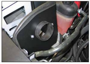
18. Install the filter adapter onto the heat shield and secure with the provided hardware.
