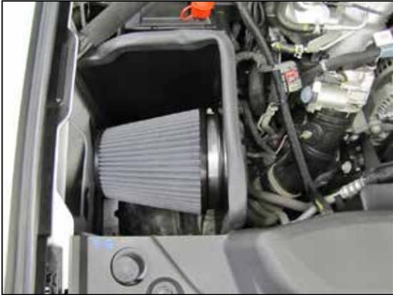
9. Flex the heat shield inward towards the engine then install the air filter onto the filter adapter and secure with the provided hose clamp. Secure the heat shield with two of the remaining factory bolts from step #5.
