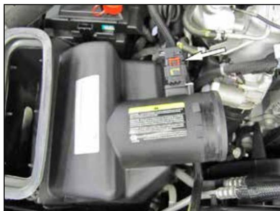
4. Release the red locking tab and then disconnect the mass air sensor electrical connection. Unhook the coolant bypass hose from the air filter housing. Lift the air filter housing up to dislodge it from the mounting grommets and remove it from the vehicle.
