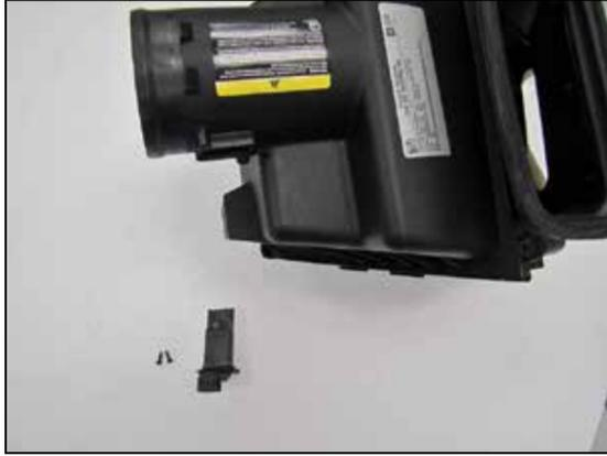
11. Remove the mass air sensor from the air filter housing.
