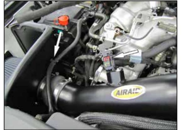
14. Reconnect the mass air sensor electrical connection and secure the coolant bypass hose to the heat shield using the factory retaining clip.
