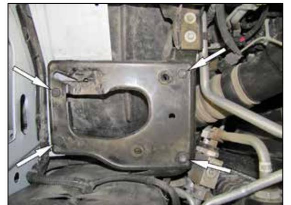
5. Remove the four bolts that secure the air filter housing mounting plate to the inner fender and then remove the mounting plate from the vehicle.
