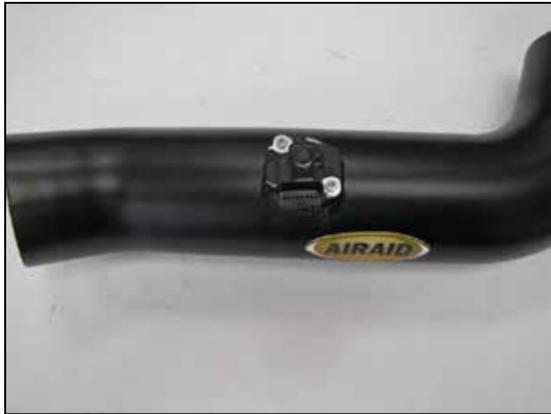
12. Install the mass air sensor into the AIRAID intake tube and secure with the provided hardware.
