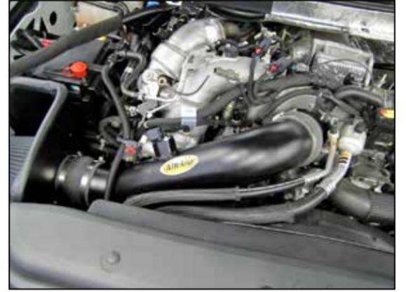
13. Install the intake tube into the coupler installed onto the filter adapter and then into the coupler installed onto the filter inlet. Adjust the tube for best fit and then secure with the provided hose clamps.
