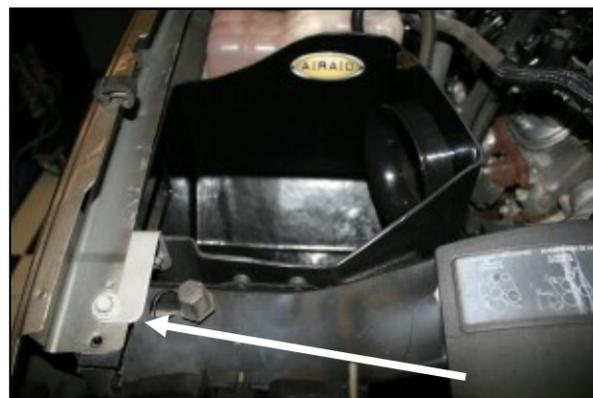
8. Install the CAB assembly into the vehicle where the factory airbox used to be using three 6mm hex bolts (#12) and three flat washers (#11) thru the bottom. Now reinstall the factory fender bolt thru the bracket and into the fender. Adjust the assembly for fit and tighten all bolts and nuts at this time.
