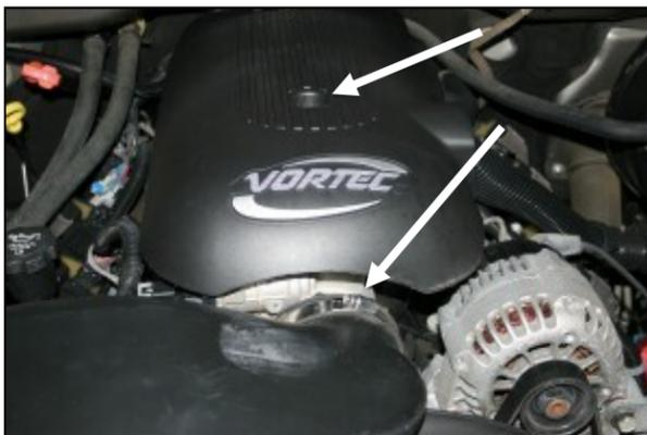
1. **Disconnect the negative battery cable.** Loosen the bolt that secures the battery cover to the engine and remove it and the cover from the vehicle. Loosen the hose clamp that secures the factory air intake tube to the throttlebody.
