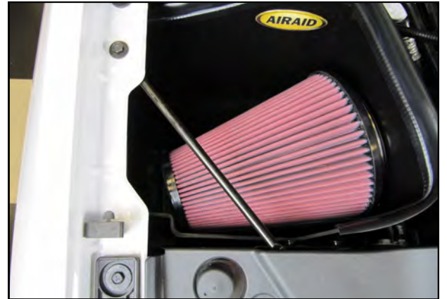
15. Reinstall the fender brace. Make sure all clamps, hoses, bolts, and screws are tight. Double check the hood clearance. Reconnect the negative battery cable.
