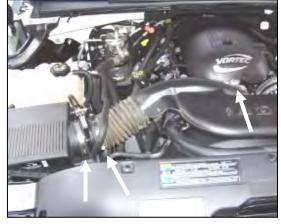
1. <u>Disconnect the negative battery cable.</u> Loosen the hose clamps located at the Mass Air Flow (MAF) sensor, and throttle body on the factory intake tube assembly.
